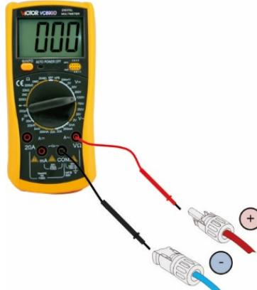
Step 5: Insert the DC connector into the corresponding DC terminal until a "click" sound is heard.
