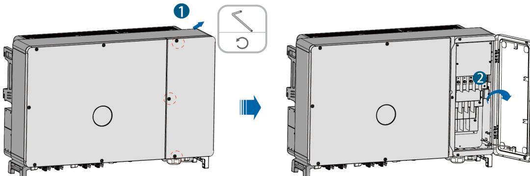
Step 3: Use the limit bar on the terminal box cover to fix its position for easy wiring operation.
