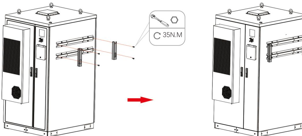
**Step 3:** Place the converter on the back plate and make sure it is properly installed; Then tighten the following two M6\*16 screws on the side to ensure a firm connection between the converter and the battery cabinet.
