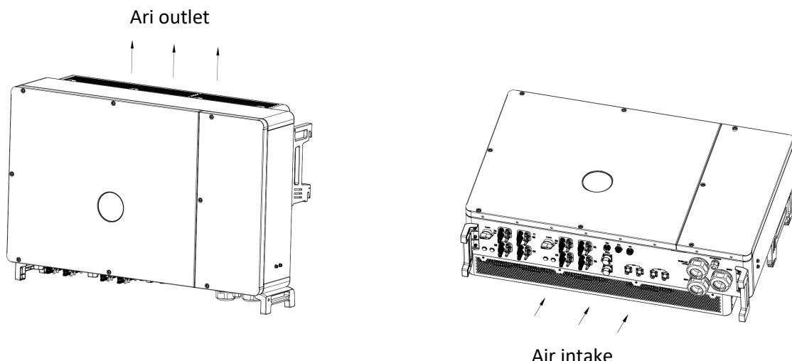
Figure 5-7 Schematic Diagram of Air Inlet and Outlet
