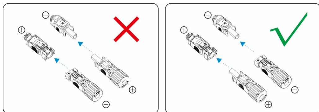
Before connecting the DC connector to the inverter, check the positive and negative polarity of the battery board
