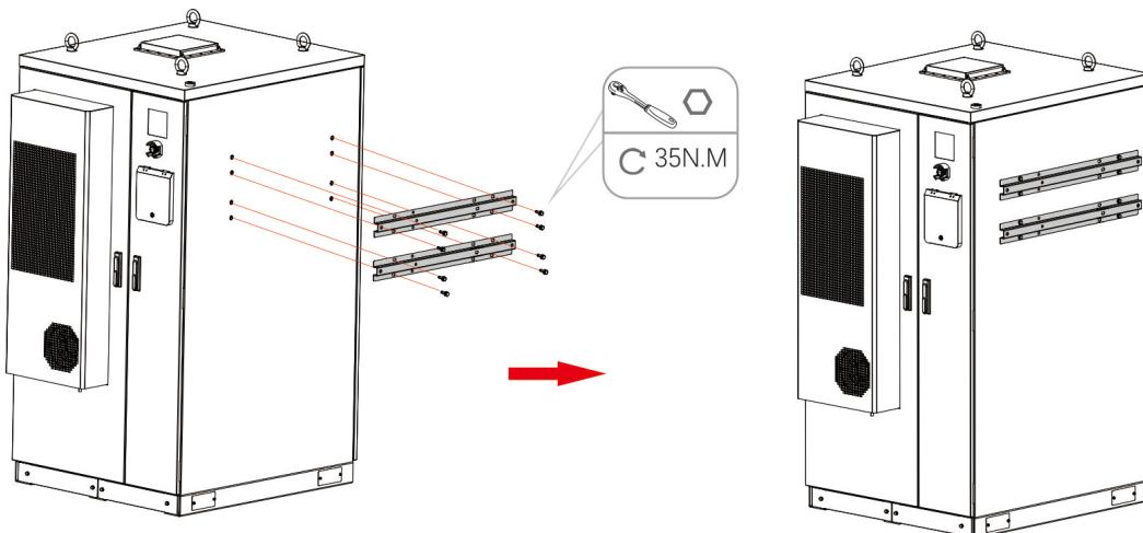
**Step 2:** Take out the converter back plate\*1 and M10\*30 screws\*4, and fix the back plate to the beam.
