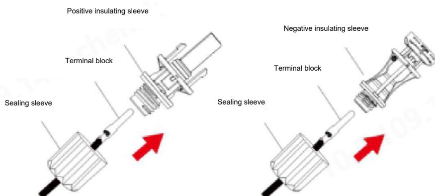
Step 4: Connect the positive and negative poles of the PV array to the "PV+" and "PV-" terminals.
