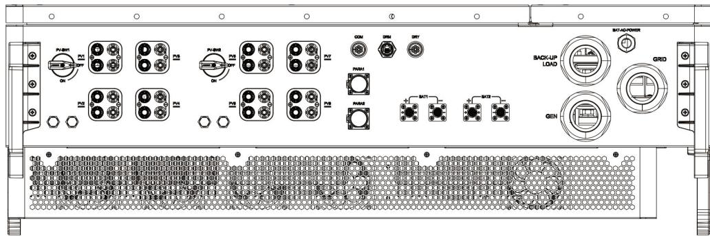
Figure 6-1 PV Connection Terminal 8-way
