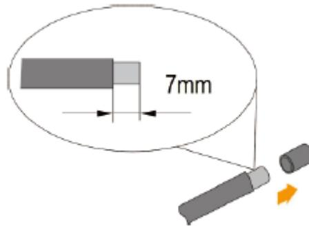
Step 2: Cluster the cable ends to the wiring terminals with crimping pliers.
