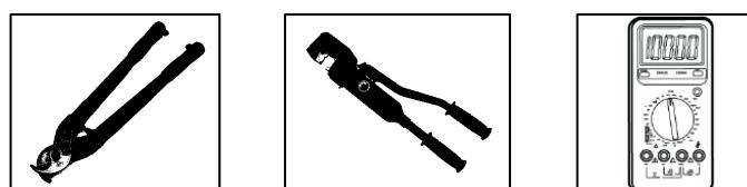
Wire stripper Crimping plier Multimeter
