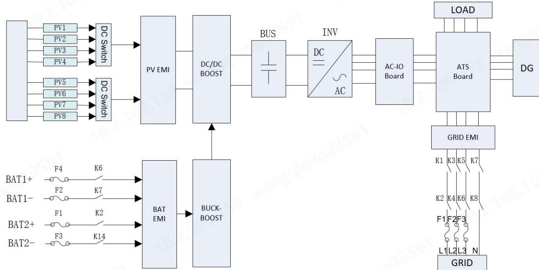
Figure 3-3 Main Circuit Topology of MF-GREENH125K
