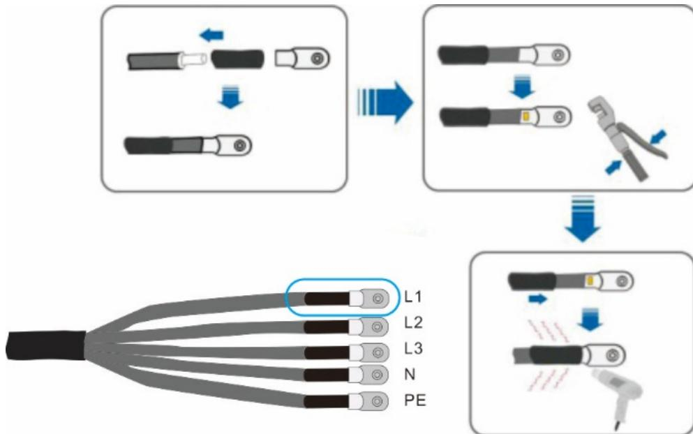
**Step 6:** Secure the cables to the corresponding terminals.
