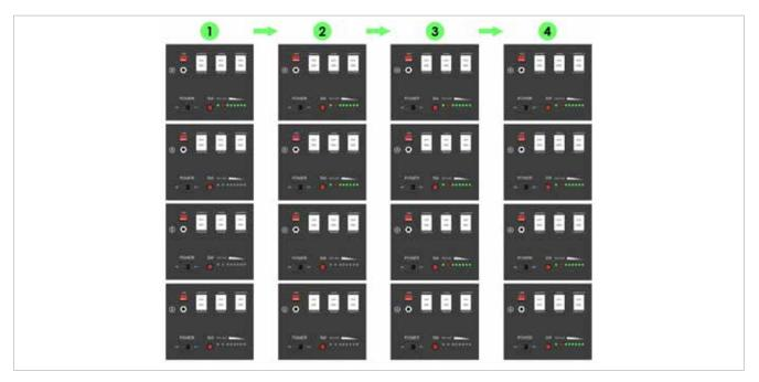
3) Press the red SW button of master battery to power on, all the battery LED light will be on one by one from the Master battery:
