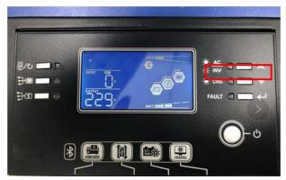
(c) Press 'Up' and 'Down' to choose the setting item No., press 'Enter' to enter into the detailed setting parameter, when finish press 'Enter' again. The following setting items need to be set follow the recommended value:
