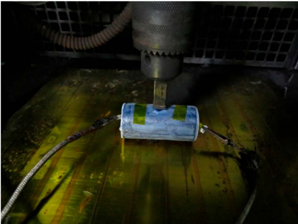
Figure 4 View of the internal short-circuit location
