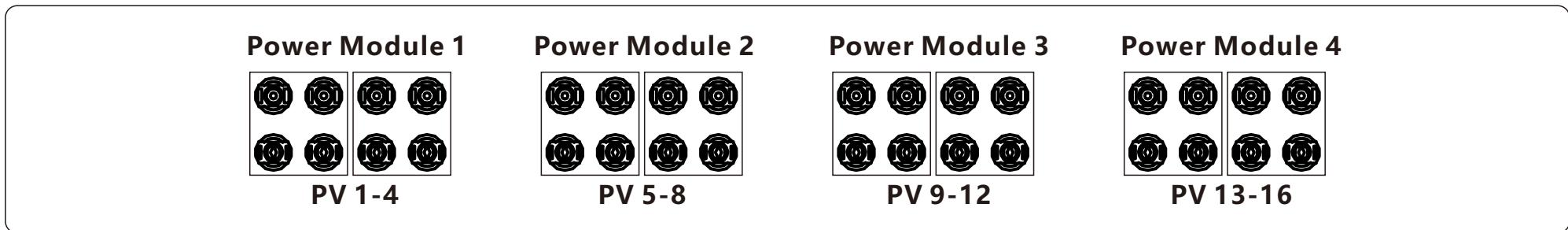
If four power modules are indeed required to connect the solar panels unevenly, for a power module which is connected to four strings, it is necessary to ensure that the power of each PV strings connected under this power module does not exceed 8.5kW to achieve better power generation performance. In the case that the power difference between each PV string is less than 10%, the 3 common cases are showing below.
