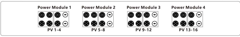
If four power modules are indeed required to connect the solar panels unevenly, for a power module which is connected to three strings, it is necessary to ensure that the power of each PV strings connected under this power module does not exceed 11.3kW to achieve better power generation performance. In the case that the power difference between each PV string is less than 10%, the 3 common cases are showing below.
