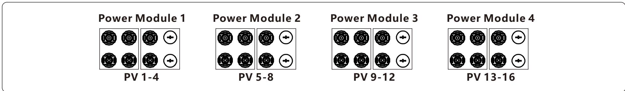
If four power modules are indeed required to connect the solar panels unevenly, for a power module which is connected to three strings, it is necessary to ensure that the power of each PV strings connected under this power module does not exceed 11.3kW to achieve better power generation performance. In the case that the power difference between each PV string is less than 10%, the 3 common cases are showing below.
