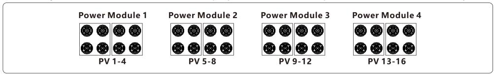
If four power modules are indeed required to connect the solar panels unevenly, for a power module which is connected to four strings, it is necessary to ensure that the power of each PV strings connected under this power module does not exceed 8.5kW to achieve better power generation performance. In the case that the power difference between each PV string is less than 10%, the 3 common cases are showing below.
